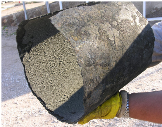
Figure 10: Silica based scaling in the Tuzla Power Plant
