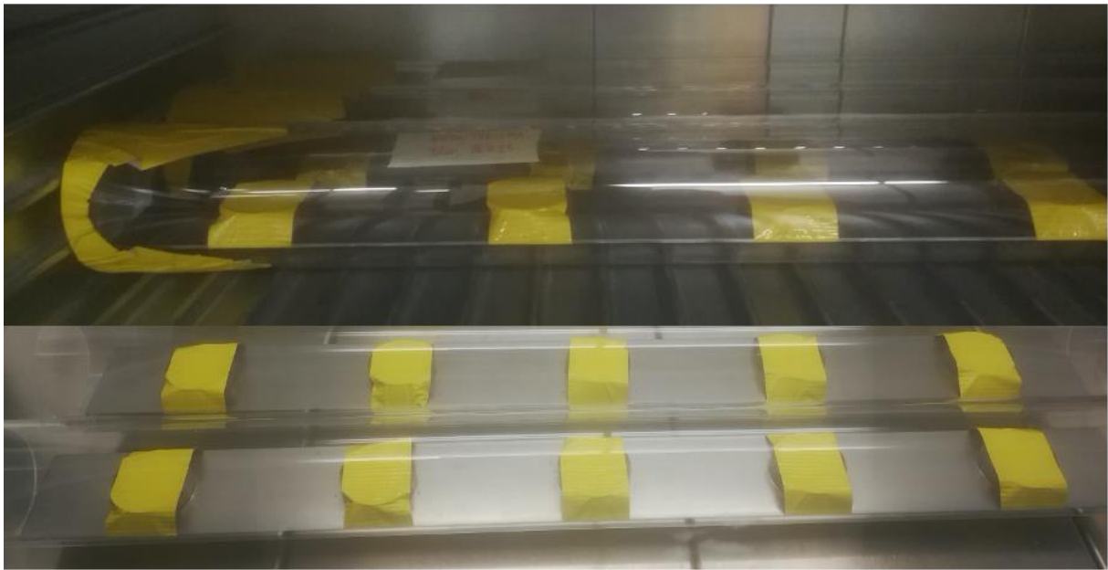
Figure 35: Images showing the setup use for the production of complex biofilms on 80cm steel plates. Ongoing incubation of P. citrinum in MA-filled Petri dishes on 80cm steel plates placed in the incubator at 30°C.
