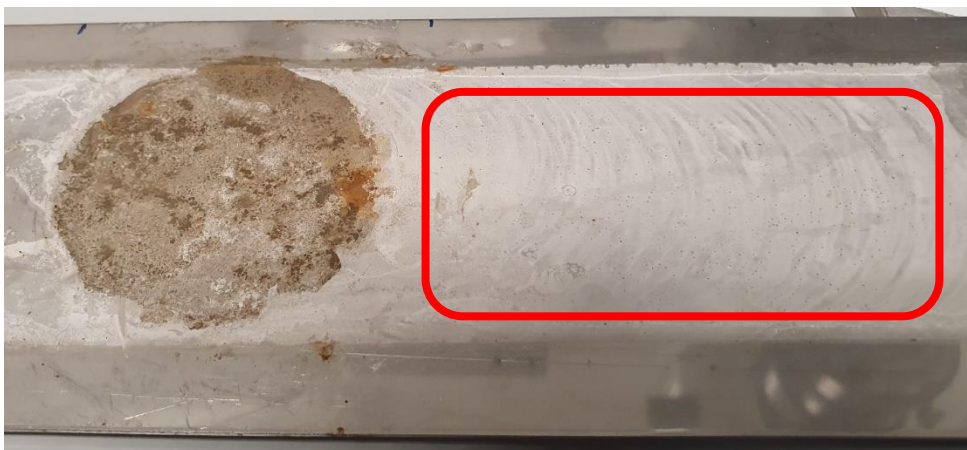
Figure 50: Picture of the sample used in the flow-loop set-up after performing the experiment. Extensive scaling deposition (red encircled area) on blank steel areas are clearly present.
