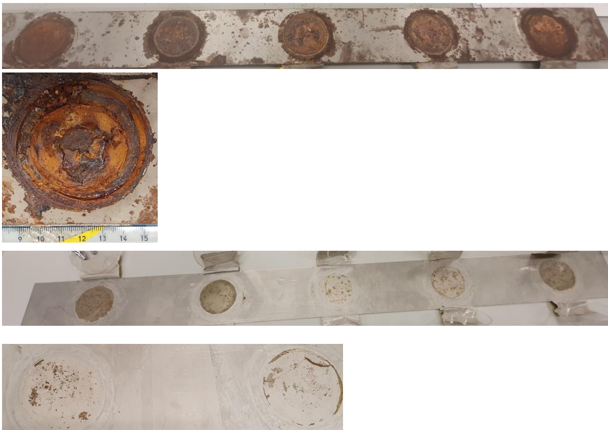
Figure 36: Examples of the biofilms on steel substrates to be used in the large flow-loop set-up as supplied by Kilian Blaise (UNINE). Extensive corrosion occurred (a, top images) as shown in the top images. Example of the biofilms on steel substrates used in the large flow-loop set-up as supplied by Kilian Blaise (UNINE; b, bottom images).
