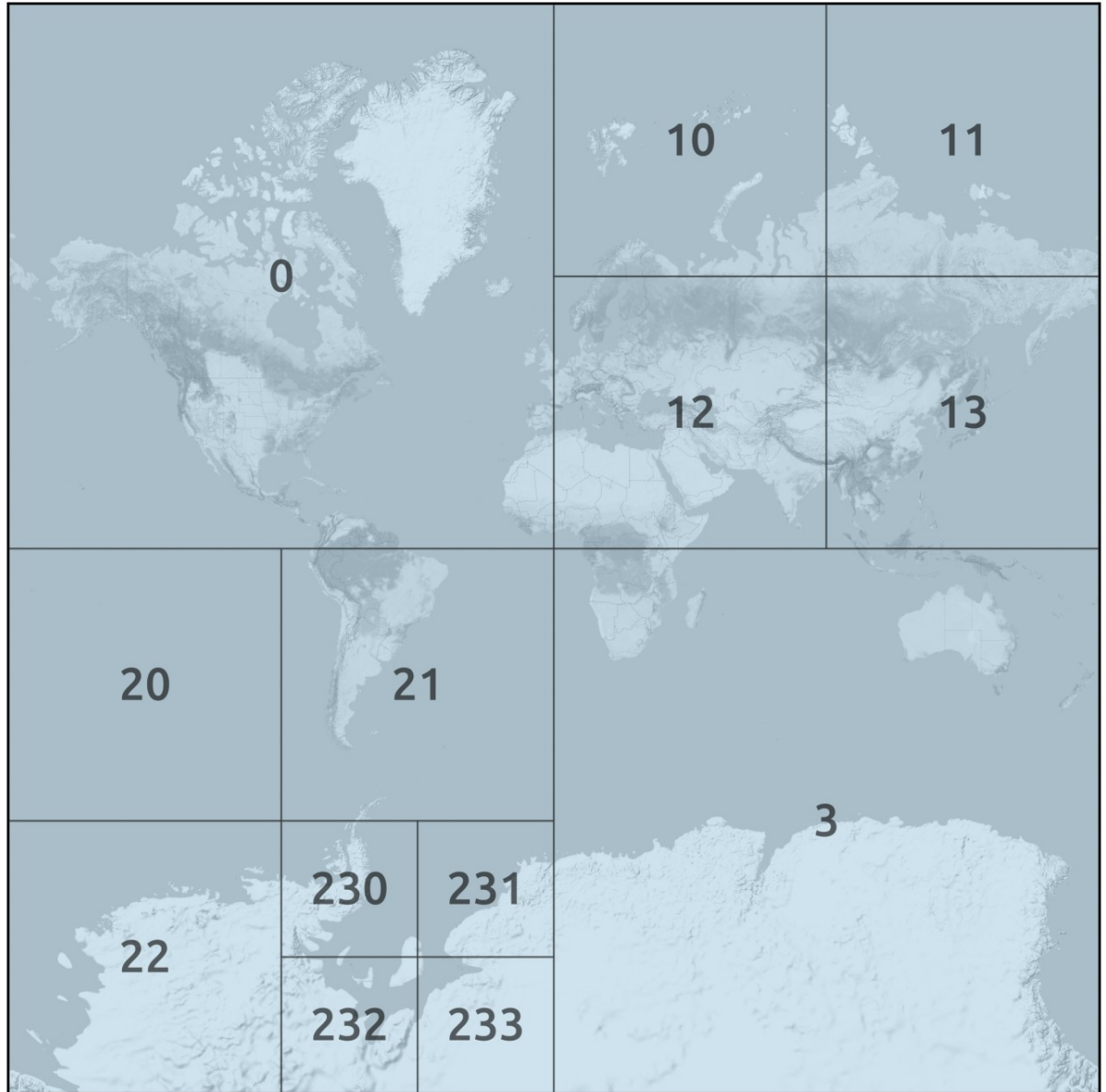
Figure 2. Quadtree-based recursive division of the globe into tiles at various zoom levels. Map tiles by Stamen Design under CC BY 3.0. Data by OpenStreetMap and contributors under ODbL. Modified from original.
