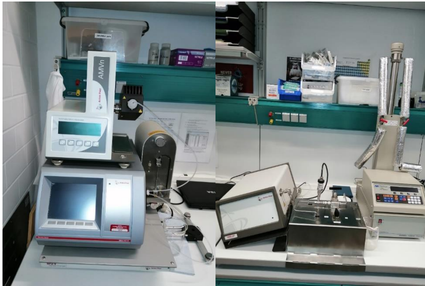
Figure 18. - Density measurements. Left: Anton Paar DMA4500M for measurements at ambient pressure; right: DMA-HP.
