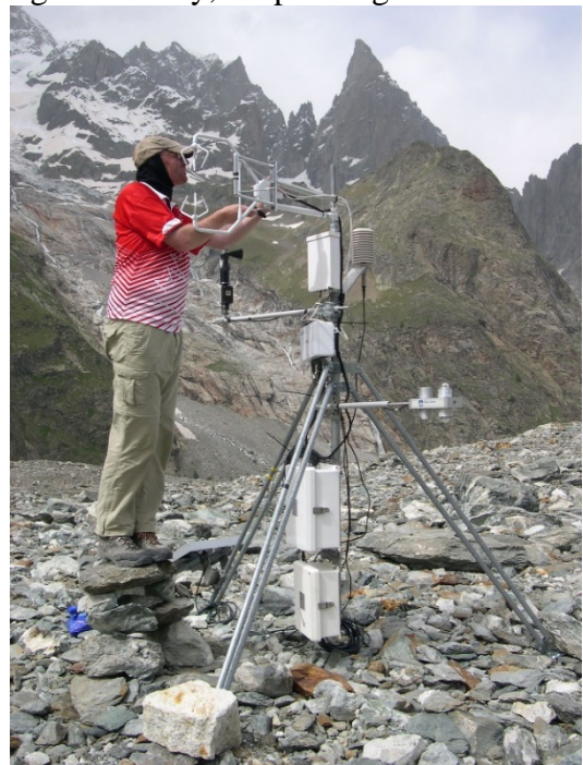
Installing eddy-covariance instruments on the debris cover of the Miage glacier, Italy
