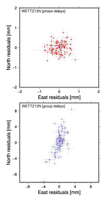
Figure 5. Residuals of the position estimates of antenna WETTZ13N in the horizontal plane from group delays (bottom) and phase delays (top) in the 107 global 24-hr sessions. The residuals in both plots are relative to the weighted mean position from phase delays. The weighted mean of the residuals is marked as a purple dot in both plots. Note the different scale.
