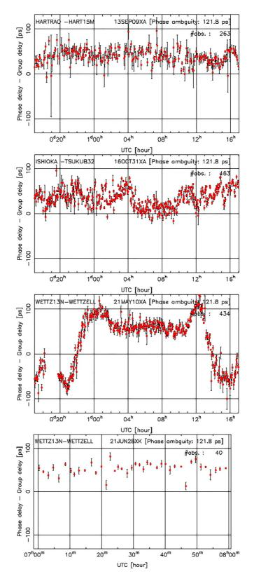
Figure 2. Demonstration of the differences between group delays and phase delays for baselines HARTRAO-HART15M (top), ISHIOKA-TSUKUB32 (middle top), and WETTZ13N-WETTZELL (middle bottom) in 24-hr sessions and for baseline WETTZ13N-WETTZELL in a 1-hr session (bottom). Error bars shown are the combined uncertainties of the phase delays and the group delays. The plotting scale corresponds to about minus and plus one turn of phase.
