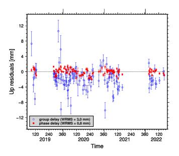
**Figure 4.** Residuals of the estimated Up coordinates of antenna WETTZ13N from group delay observables (blue open circles) and phase delay observables (red closed circles) based on geodetic analyses of 107 global 24-hr sessions. The error bars are the formal errors of the estimates from geodetic analyses.
