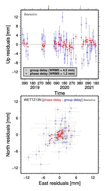
Figure 6. Residuals of the Up component (top) and the east and north components (bottom) of WETTZ13N position estimates from 58 Intensive sessions, relative to the weighted mean position from phase delays in 24-hr sessions reported in Table 2. Note the different scale compared to the residual scatter shown in Figure 5.
