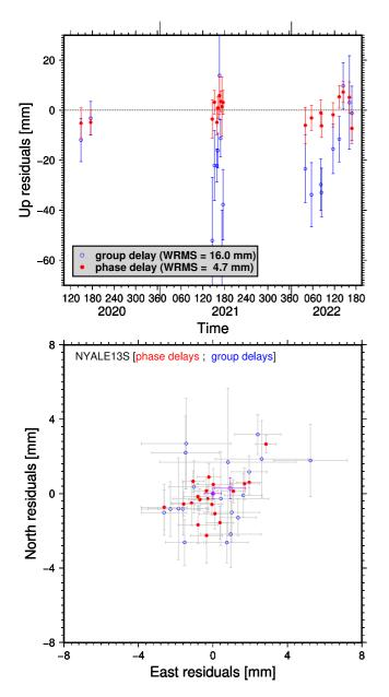
Figure 7. Residuals of the Up component (top) and the east and north components (bottom) of NYALE13S position estimates. The residuals are drawn by blue open circles for group delay results, and by red closed circles for phase delay results. The weighted means of the residuals are marked as purple dots in the bottom plot.
