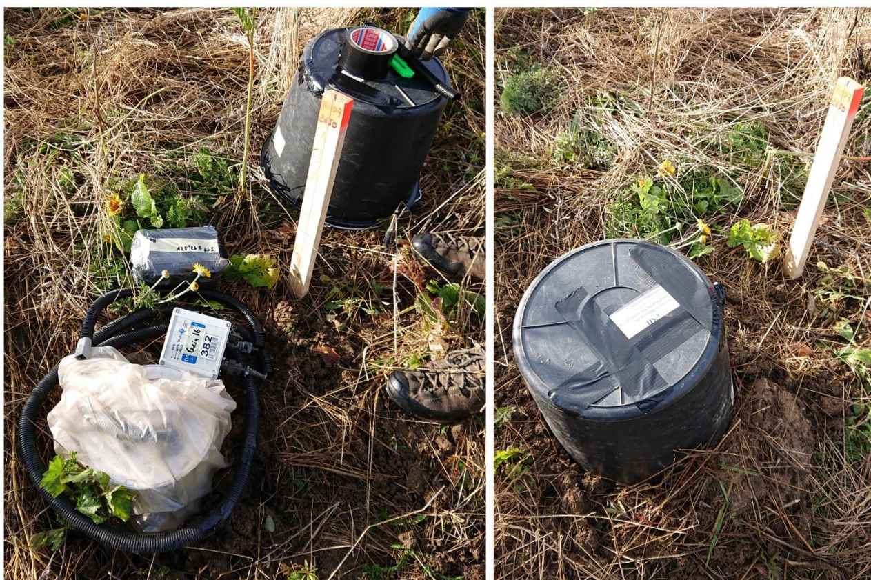
Figure 2: Exemplary instrument installation at recording site IW05H. The sensors and the battery boxes were protected with plastic bags against moisture and the sensors were buried to a depth of about 20 cm (MARK instruments) or 30 cm (Trillium Compact instruments). The Trillium Compact sensors were additionally fixed to the ground with fast-drying cement to ensure stability. Plastic cable protection was used against rodents for all cables. Left: Buried MARK sensor inside a plastic bag. The CUBE3 data logger and the battery box are located at the surface. Right: The site after the installation.
