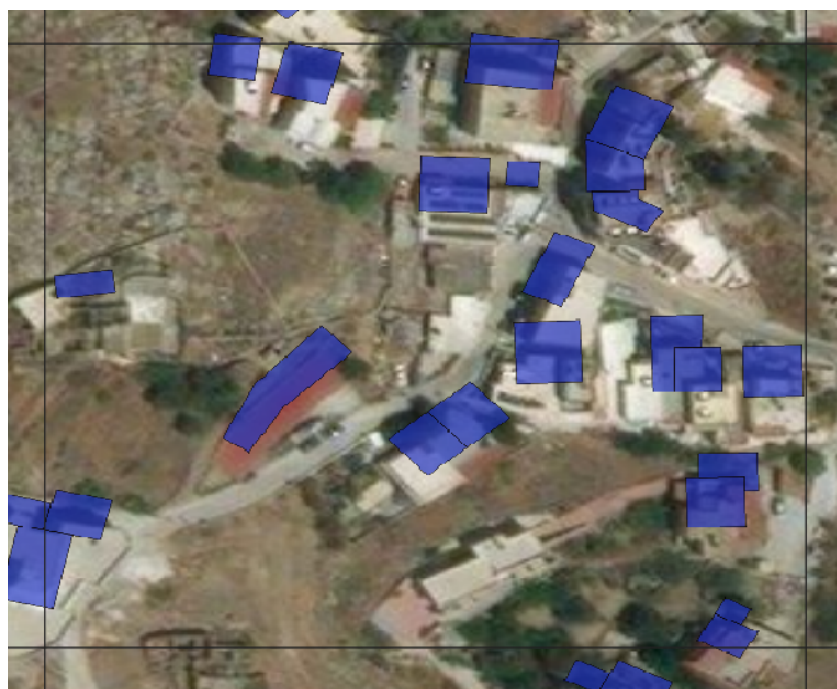
Figure 5. Example for a misalignment of the OSM building footprint layer and satellite imagery. The example is taken from the case study at Sirios.
