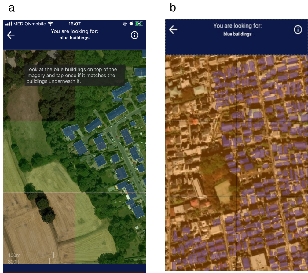
Figure 1. MapSwipe main screen. Two examples are given: (a) Green-colored tiles represent complete tiles, untapped tiles represent no building tiles; (b) Orange-colored tiles represent areas that are incompletely mapped in OSM with respect to building footprints.
