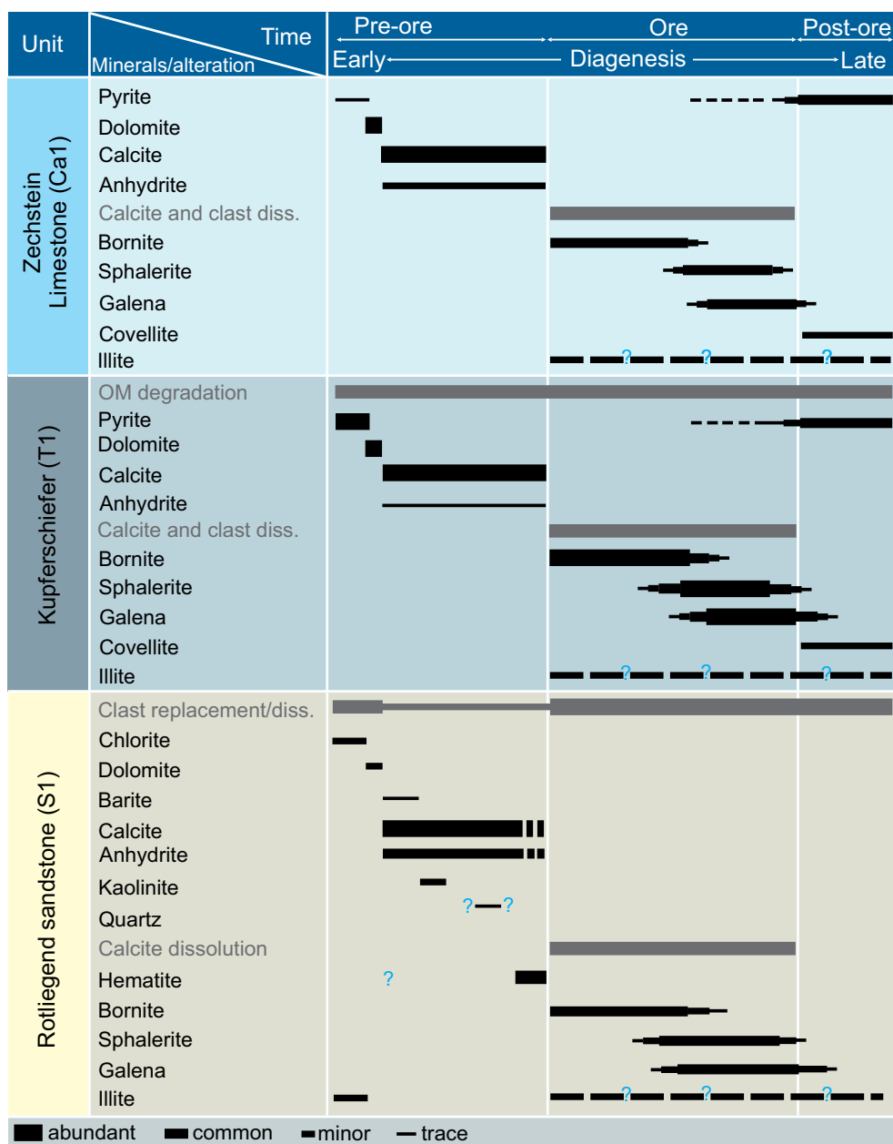
Fig. 3. A paragenetic chart for the mineral phases in the Rotliegend sandstone (S1), Kupferschiefer (T1), and Zechstein limestone (Ca1). diss = dissolution, OM = organic matter.
