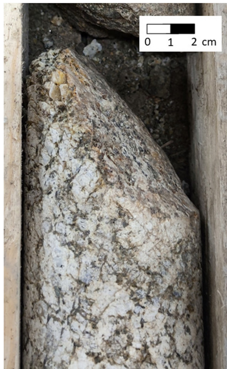
Figure 6. The S4b drill core (granite) at the depth of 140.5 m. It shows the maar-diatreme contact with the granites along a sharp plane dipping 68° from horizontal (measured by clinometer) distinctly visible on the granitic core sample.
