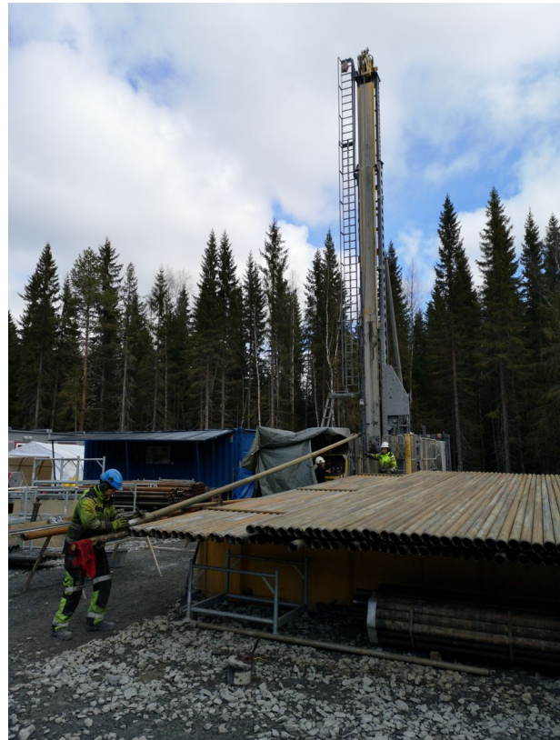
Figure 3: Riksriggen with the manual rod handling system on top of the mud tanks.
