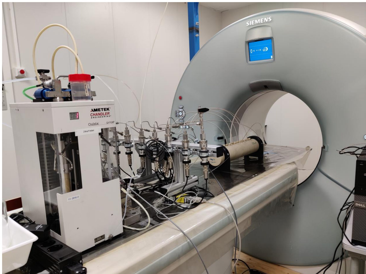
Figure 2: Photograph of the coreflooding setup in the CT scanner
