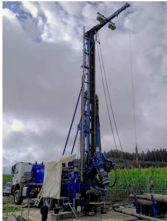
Figure 2: The drill rig (MB Actros 3341A, UH2) used for all three boreholes, with the manual casing handling system.
