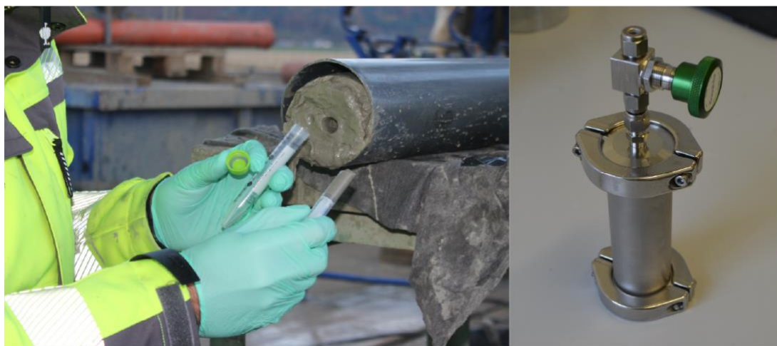
Figure 15: Left, taking a bio sample from the core. Right, vessel used to store samples for noble gas.
