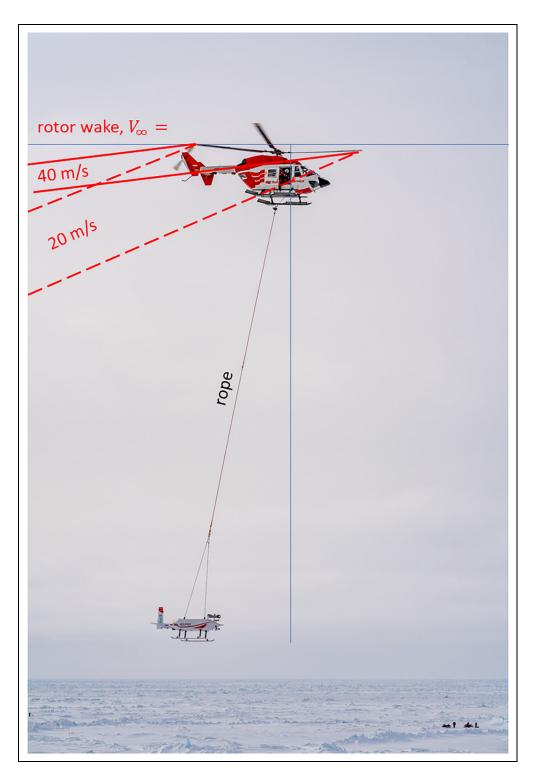
Figure 1. HELiPOD after takeoff during MOSAiC with illustration of the rotor downwash area for the measurement speed of 40 m s<sup>-1</sup> and for an airspeed of 20 m s<sup>-1</sup>. Picture: C. Rohleder.
