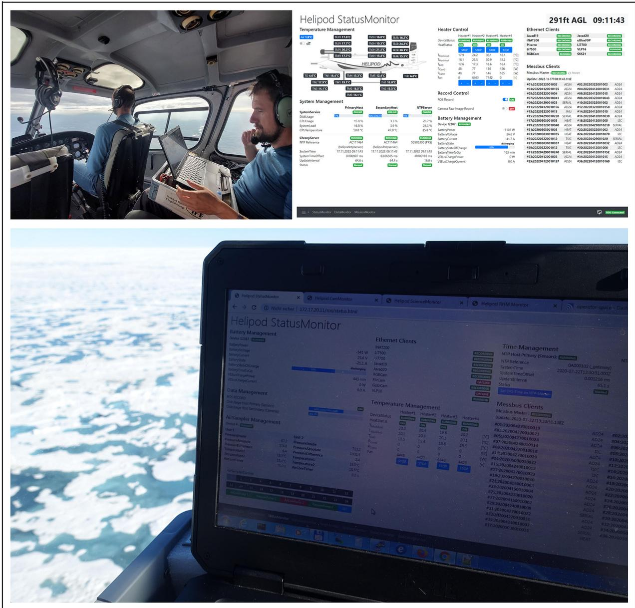
**Figure 8. Remote WiFi access to the HELiPOD during flight.** A specially developed user interface enables to monitor the current state of the whole system and sensors. Live sensor data are displayed allowing operational decision-making. A control of sensors and temperature management is given.
