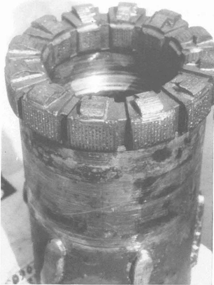
Fig. 4 High performance impregnated diamond core bit, after drilling 140m
