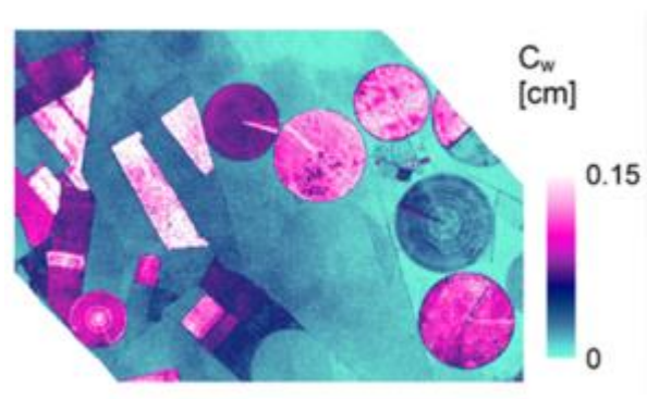
Figure 13 Exemplary map of Leaf water content (EWT, C_w ), generated using Analyze Spectral Integral (ASI) of the EnMAP-Box Agri-tools (Barrax, Spain).
