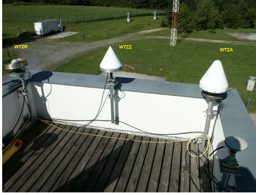
Figure 3.16: The location of three GNSS antennas at the Wettzell co-location site that was used in the comparison (Courtesy from IGS).
