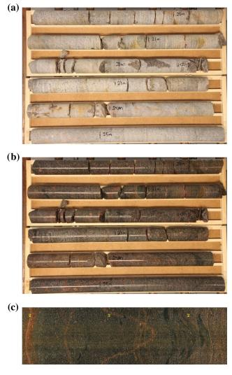
**Figure 2.** Fracture inspection from drill cores (section from 19–26 m): (a) dry, (b) wet. (c) Image from borehole televiewer BIPS tool before the experiment in the section where test HF1 was conducted (24-26 m).
