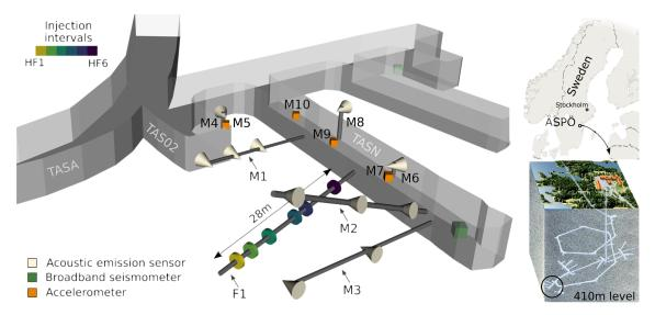
**Figure 1.** Location (top right) and overview (bottom right) of Äspö Hard Rock Laboratory with the test site at 410 m depth (left). Access tunnels are shown in lighter gray. The test borehole F1 with six hydraulic tests indicated by color and the monitoring boreholes M1–M10 with sensors (cones and cubes) are described in the following sections.
