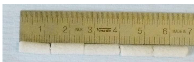
Figure 4.2. The prepared sandstone cores used in the experiments.
