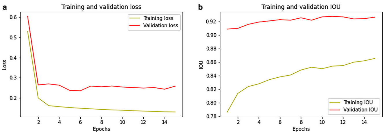
Fig. 5 a shows the progression of training and validation loss and b shows the progression of training and validation IoU for the UNet model with EfficientNet-B7 as encoder over 15 epochs
