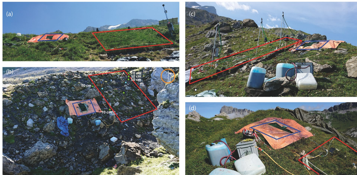
Figure 3. Examples for the positions of the dye tracer plots (blue rectangles) in relation to the isotope tracer plots (red rectangles) at three moraines at the C-PM forefield. Examples show experiments on the (a) 4.9ka, (b, c) 160a, and (d) 13.5ka moraine. (b) The positions of the soil moisture sensors (green dots), tipping bucket (turquoise dots), and weather station (orange circle).
