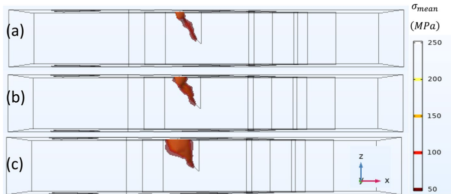
Fig. 8 Total mean stress (mean of thermoelastic and poroelastic stress) development in the geothermal reservoir after a 1 year, b 5 years and c 30 years
