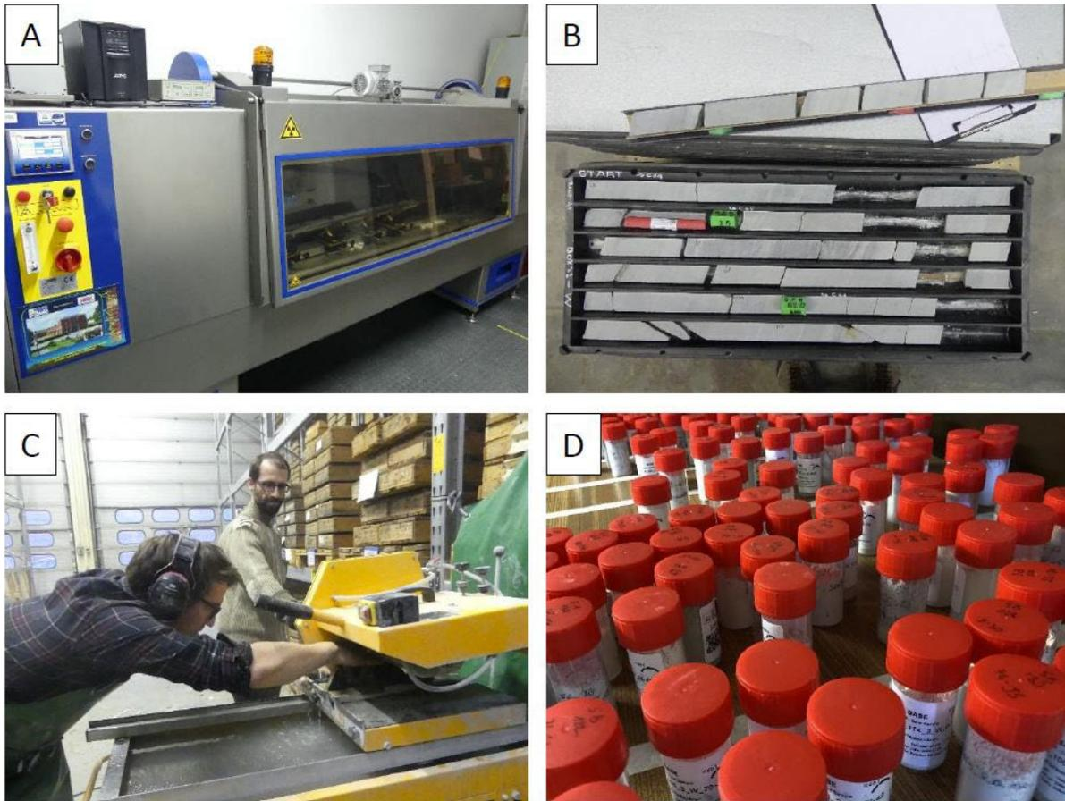
Figure 22: Producing the Geochemical Reference Data Set. A: Avatach XRF core scanner. B: Representative core tray. From each of the six grooves of this core tray, a piece ca. 10 cm long and ca. 1 m apart was removed and assembled in the portable groove to be x-rayed. Ca. 500 core trays were processed this way; all depths were documented to the mm. Red marker replaces sample taken for powder analysis. C: Cutting core halves into quarters. D: Aliquots of powdered rock samples.
