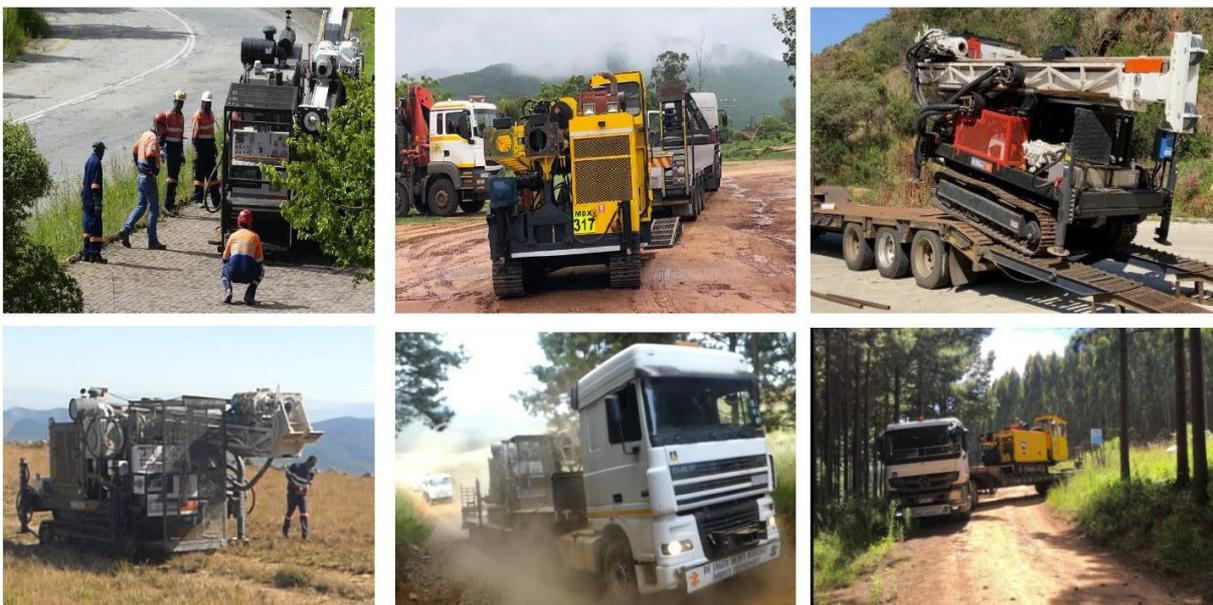
Figure 8: Drilling operations, showing offloading of the rig at drill sites, „trammelling“ between sites, and transport between sites by flatbed truck on forest dirt roads.
