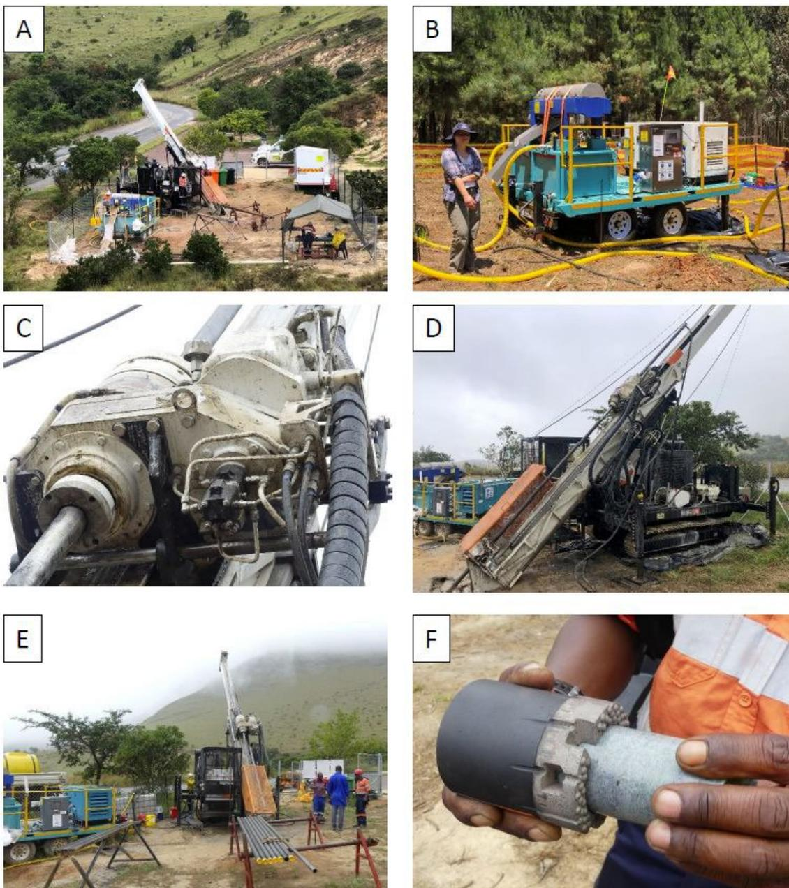
Figure 9: Drilling setup at Site 3. A. Overview; from left: bagged sludge, trailer-mounted SRU, drill rig MDX317, tressels / workbench for drill pipes, tented work area, and storage trailer. The entire site is fenced; B: Solid Removal Unit (SRU); C: „Top Drive“; D: Track-mounted drill rig; E: Site 2 overview; F: Rotary crown with piece of core.
