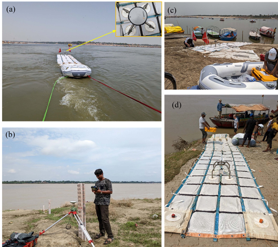
Fig. 2. Field survey conducted in Ganga river. (a) River water surface elevation measurement using GNSS carpet. (b) GCPs collection at river gauging sites. (c) and (d) field preparation.
