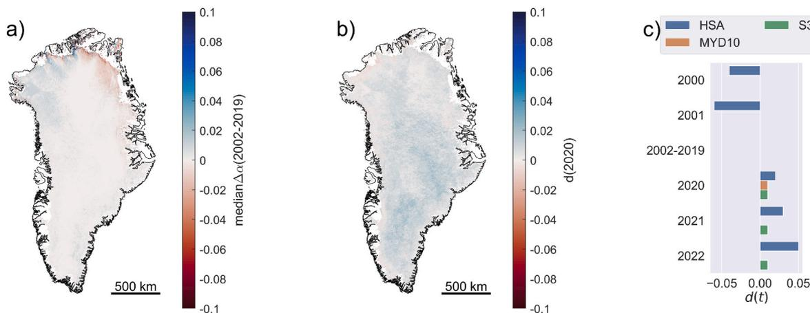
**Fig. 3.** Quantification of the orbital drift effect on MOD10. Maps of pixel-wise  $median\Delta\alpha(2002-2019)$  and  $d(2020)$  calculated using MYD10 are illustrated in sub-figures a and b, respectively. The drift effect ( $d(t)$ , subfigure c) derived from the sampling points is calculated using the HSA, MYD10, and S3 albedo.
