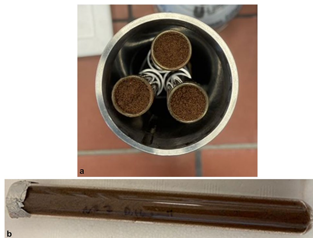
Figure 5. Images of the configuration of the exposure experiments showing (a) three sample tubes in the stainless steel sample tube holder and (b) an individual sample tube.
