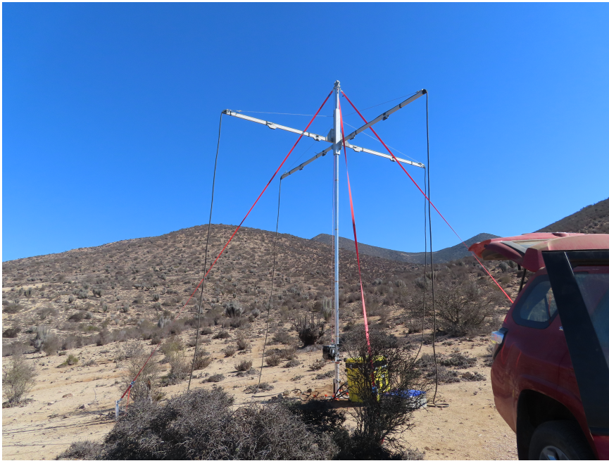
Figure 2: Horizontal magnetic dipole transmitter developed and build by Radic Research and the GFZ.
