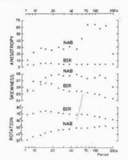
Impedance characteristics are represented for rotated coordinates, from bottom to top the rotation angle, the skewness to indicate 3-D complications, the anisotropy to indicate the degree of telluric polarization. In the foreland the rotation angle is stable and conforms with the strike of the FL ( $60^{\circ}-70^{\circ}$ ). Within the crystalline the large skewness prevents any simple interpretation of rotation angle and anisotropy which is extreme (up to 601).
