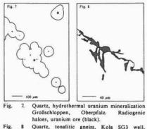
Fig. 8 Quartz, tonalitic gneiss, Kola SG3 well, depth: 11,000 m. Diffusion porosity and diffusion haloes (black).
