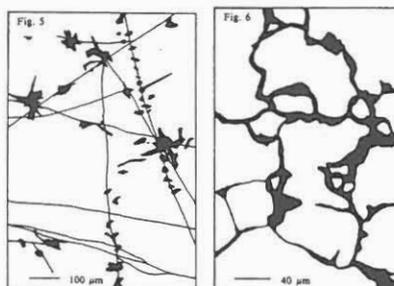
Fig. 5 Quartz, thermal crackling, Triberg granite, Schwarzwald. Pores and diffusion haloes appear black.
