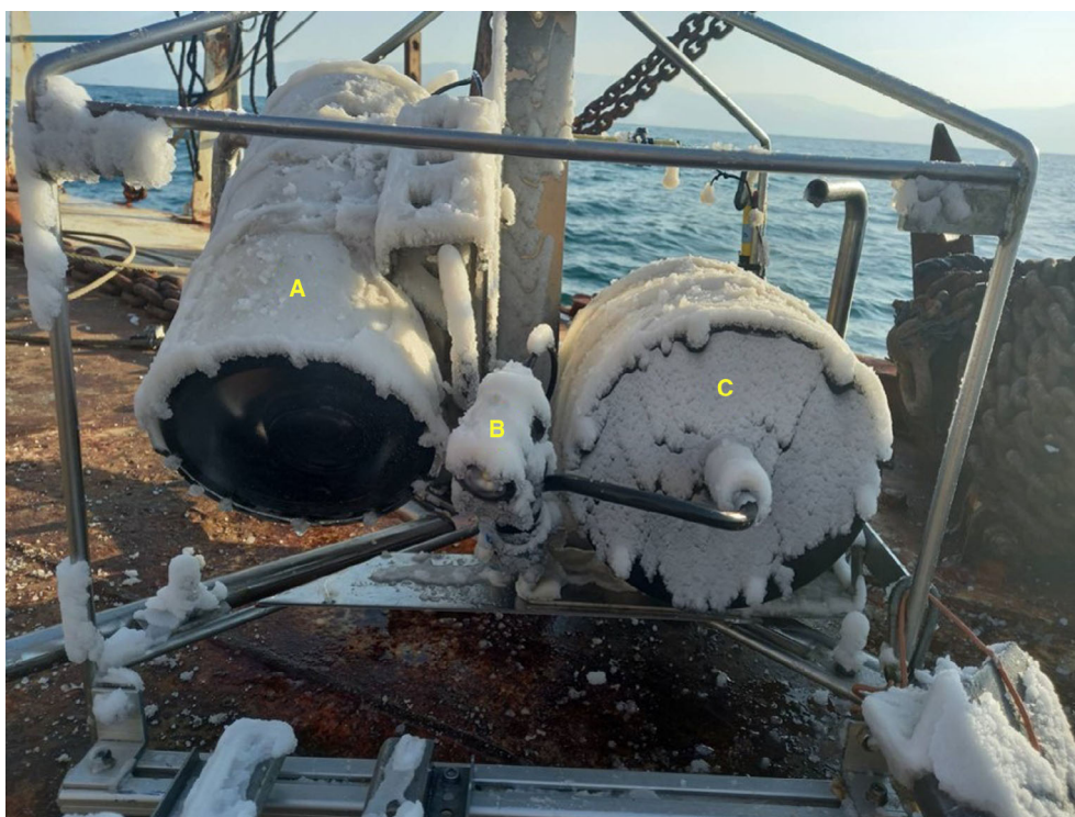
Fig. 5. The time-lapse camera device, following ten days of deployment in the mixed supersaturated brine site. The camera is covered by fine halite crystals that settle from the water column (i.e. cumulates). (A) The camera housing with the flat transparent port, (B) the flashlight and (C) the battery and controller unit in the cylindrical housing.
