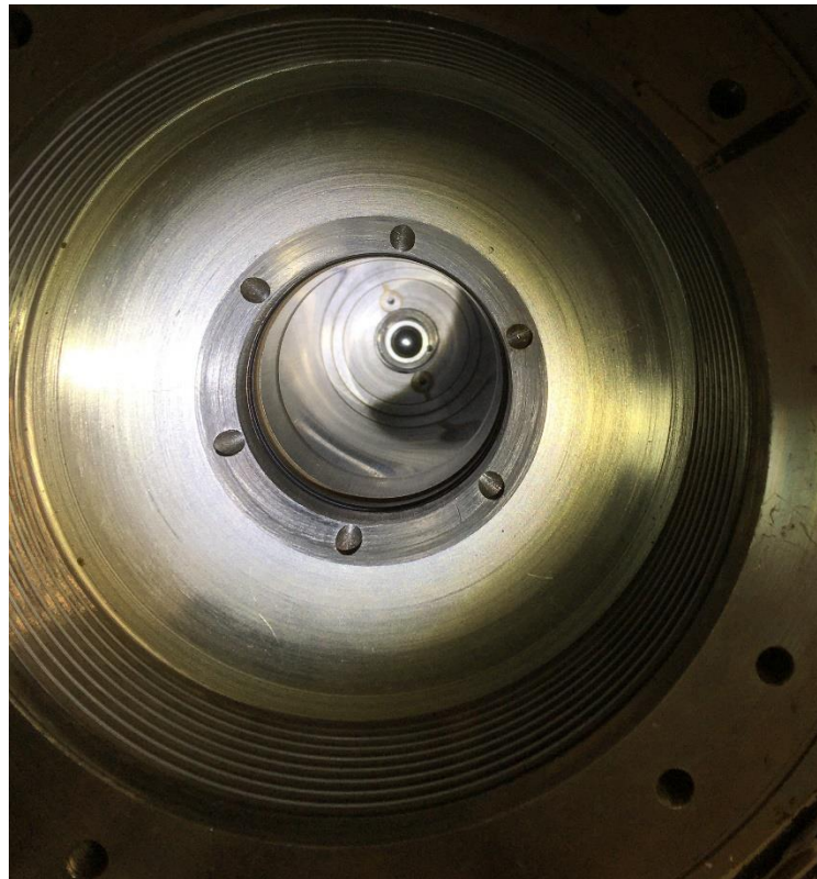
spring bottom piston in the inner anvil part of the internal load cell
