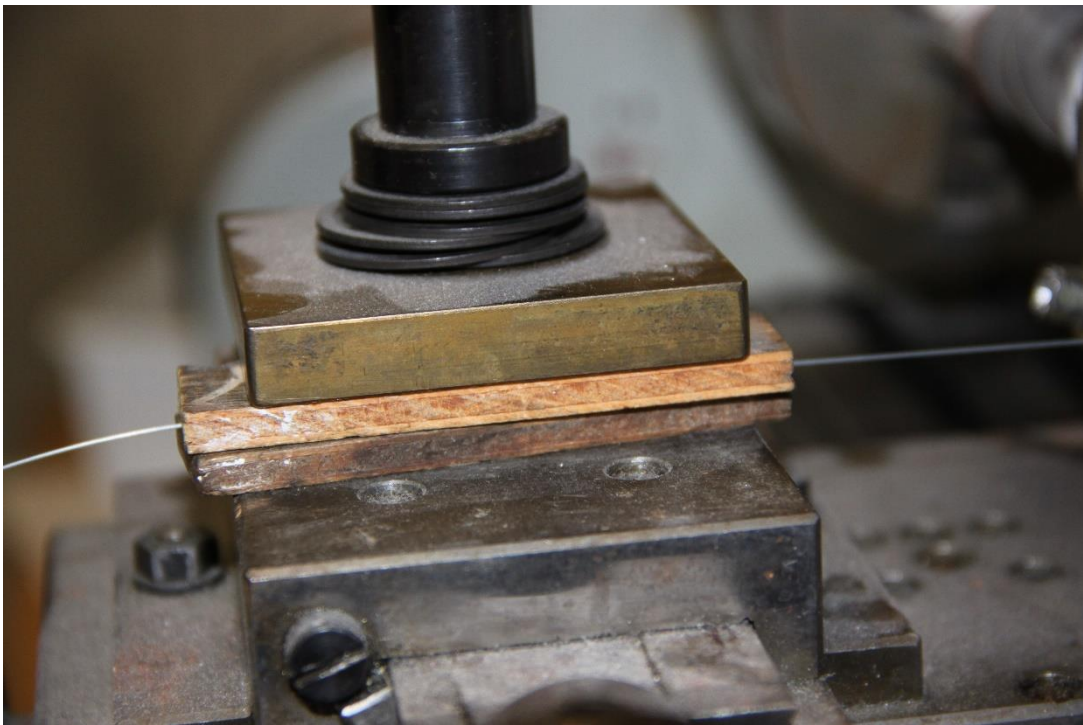
clamped winding-wire between two hard-wooden plates in the tool holder
