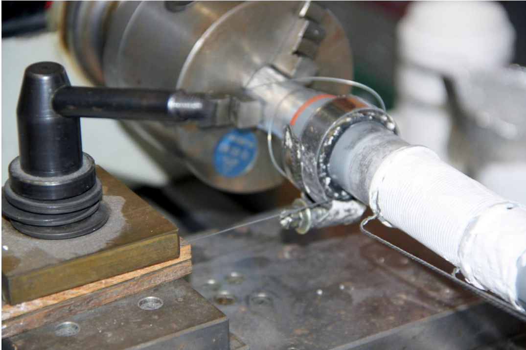
clamped winding-wire between two hard-wooden plates in the tool holder
