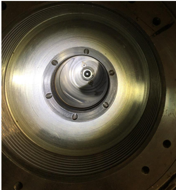
spring bottom piston in the inner anvil part of the internal load cell
