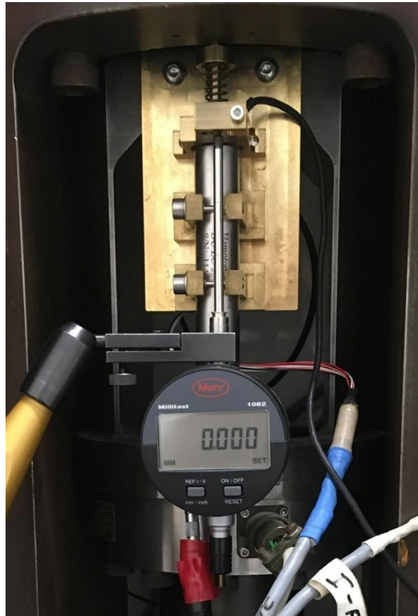
DCDT and clockwork installed at the back of the stirrup (vessel support)
