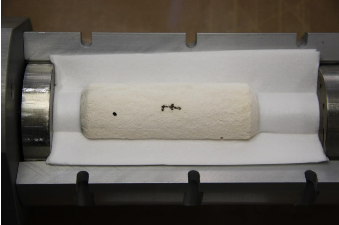
porous ceramic segment (SALI) with a layer of alumina oxide paper (APA-2) underneath
