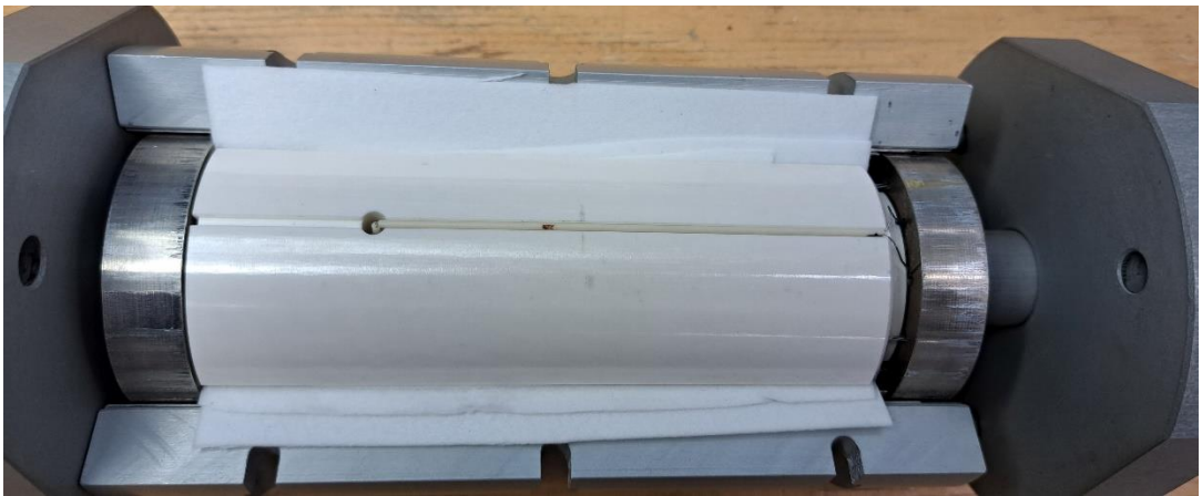
thermocouple installed completely
