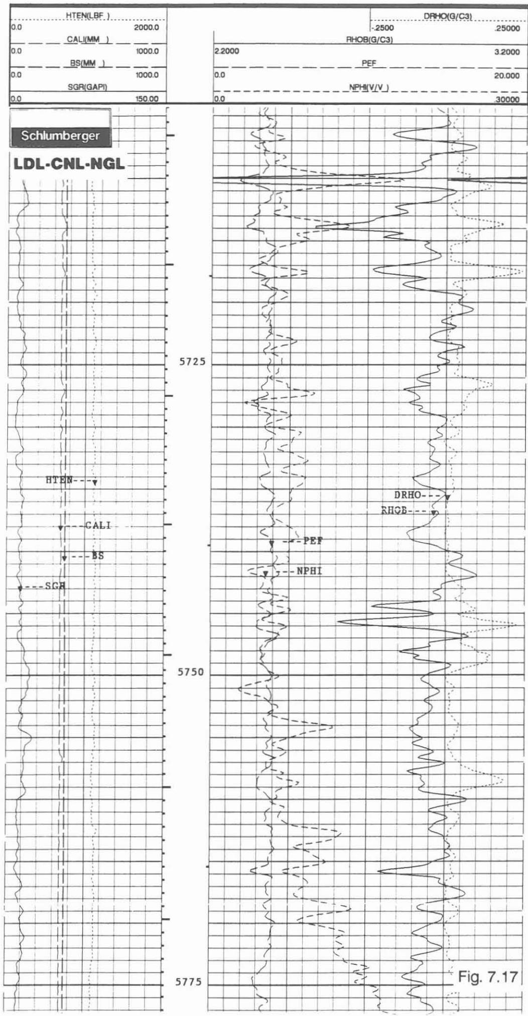
**CNL (Compensated Neutron Log - Epithermal Neutron)**
