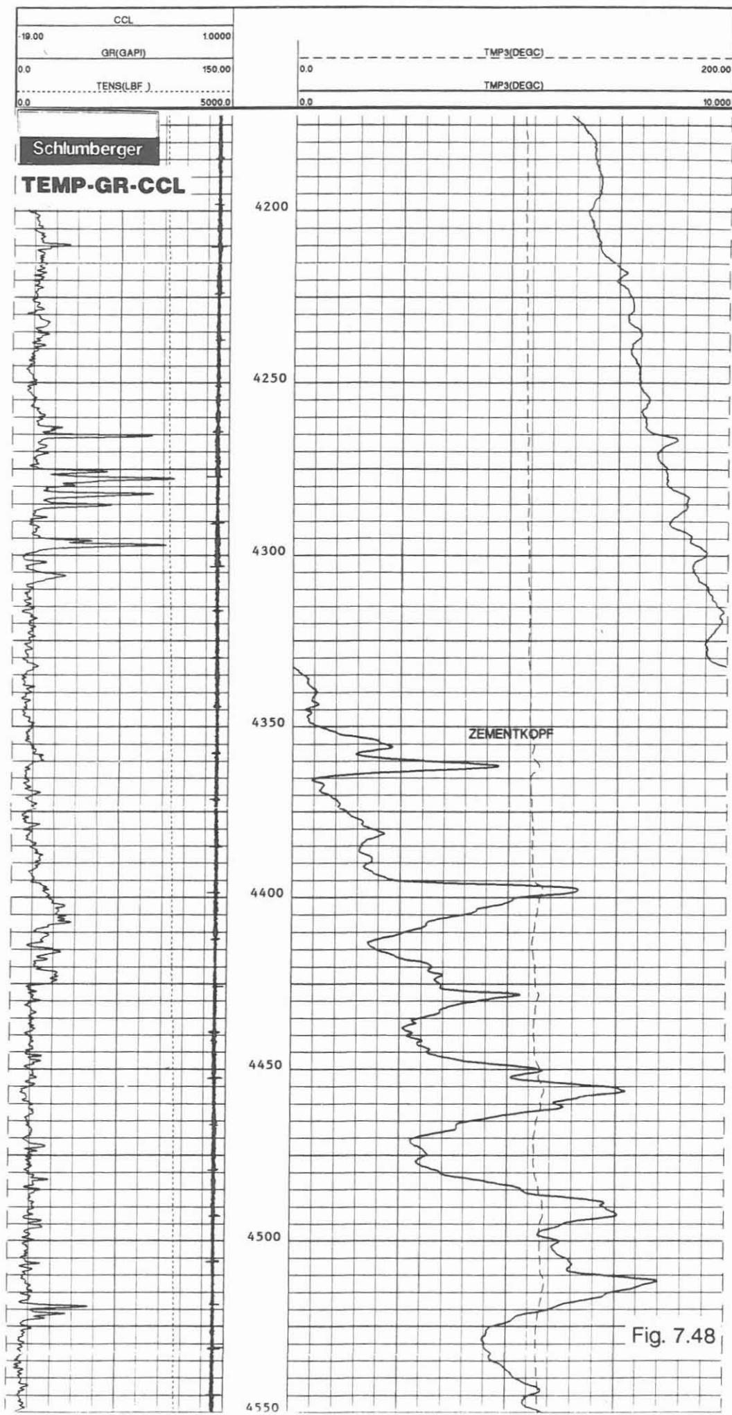
**GR/CCL (Gamma Ray/Casing Collar Locator)**
