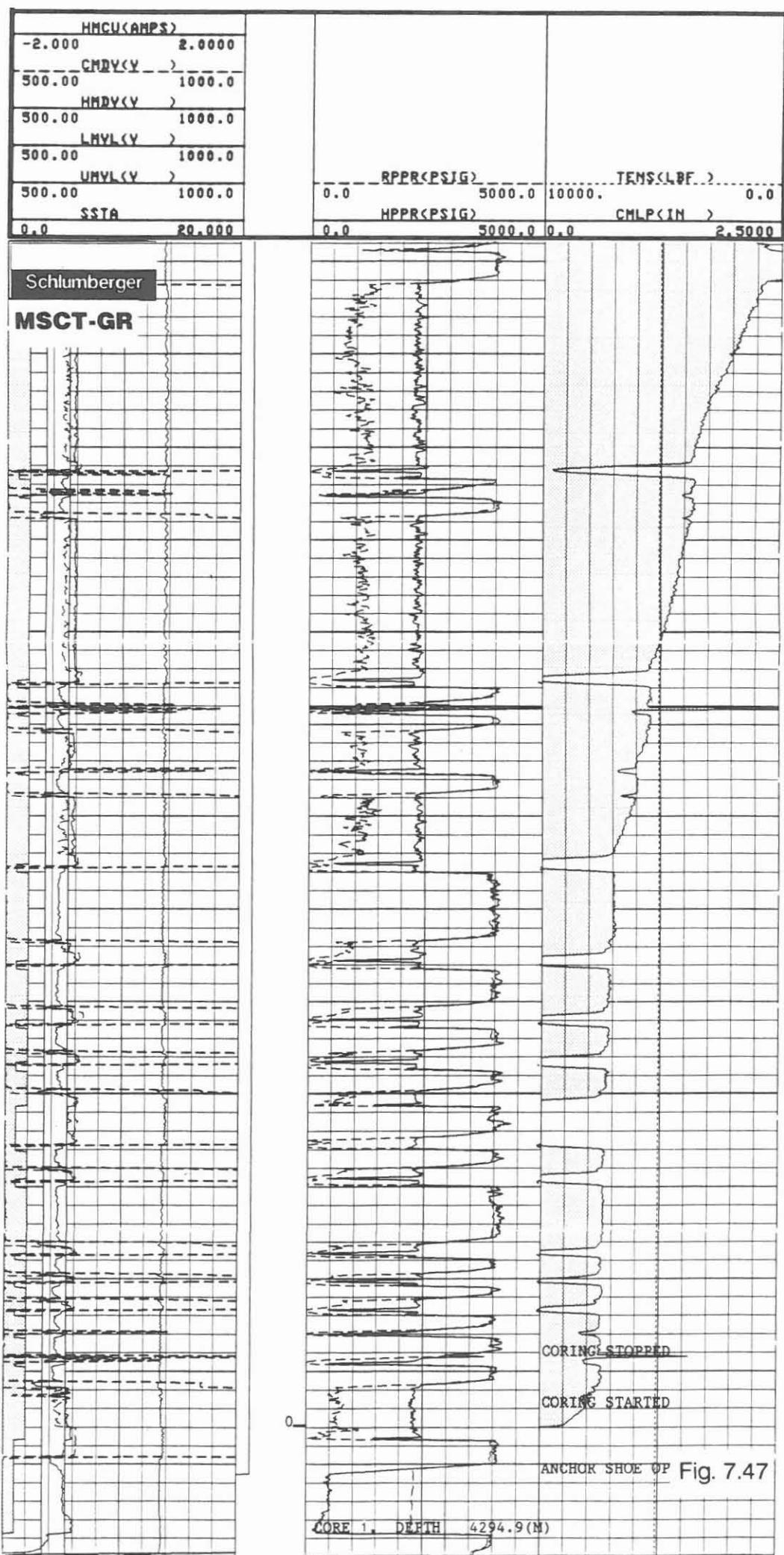
**TEMP/GR/CCL (Temperature/Gamma Ray/Casing Collar Locator)**
