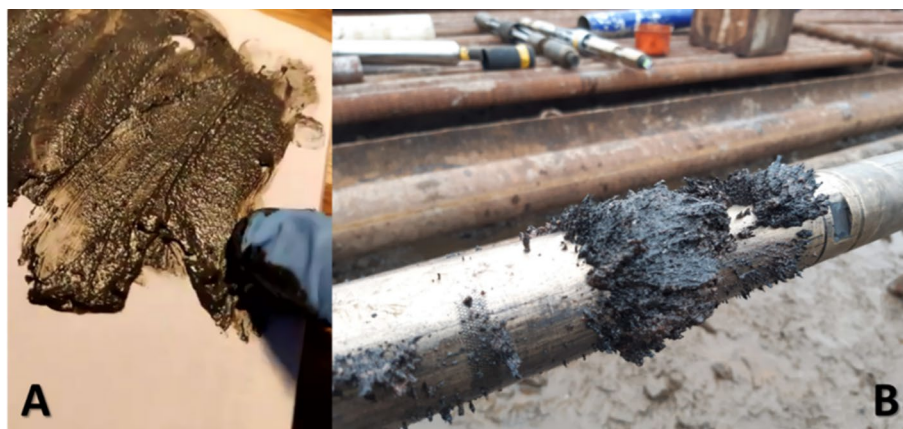
Fig. 3 Material of the bailer-collected sample (A left) and material at the downhole equipment (B right)
