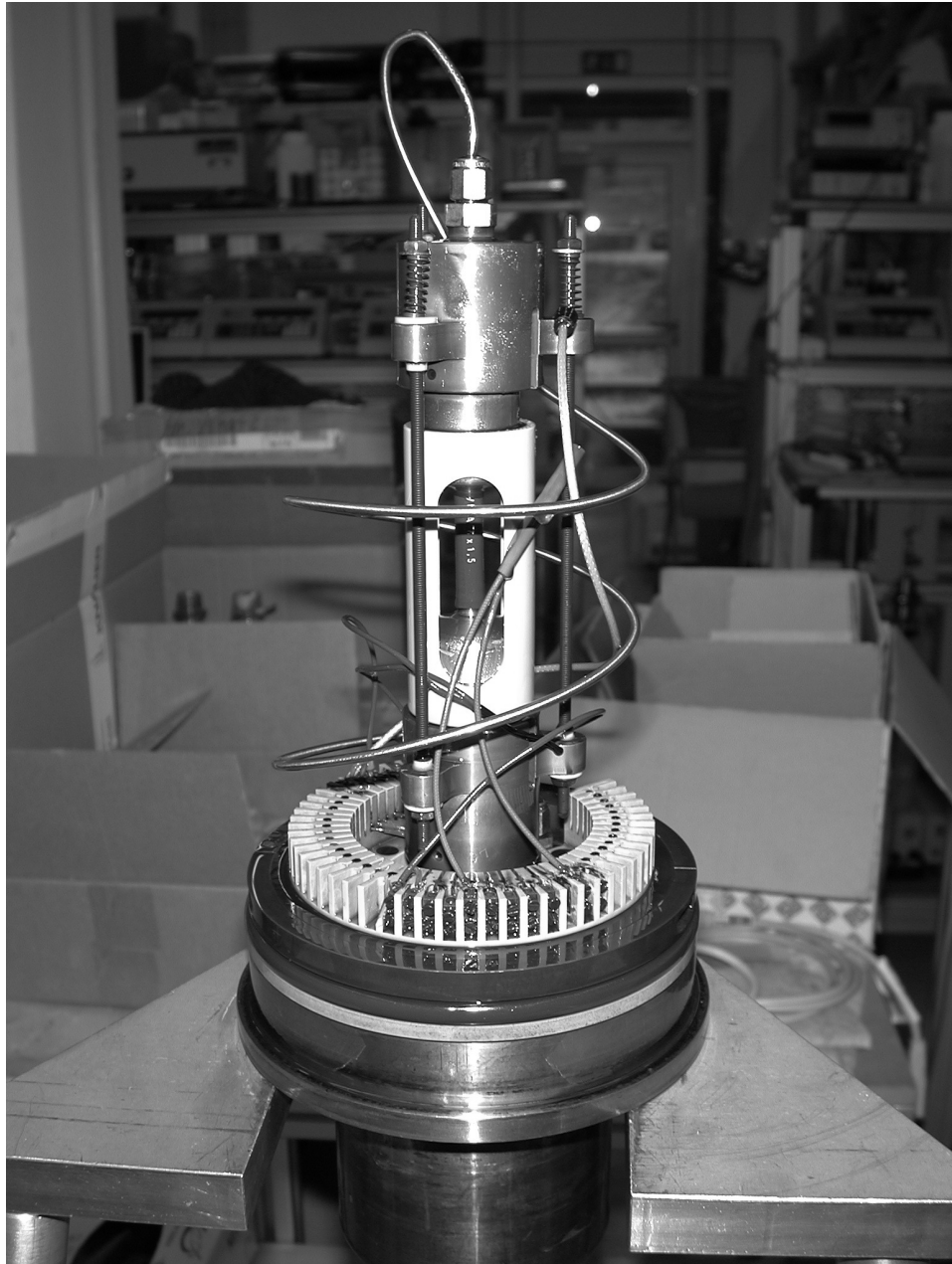
Figure 3.6: Detail of the small sample assembly (ft-F1-13). A small Flechtinger sandstone sample is located in the center of the assembly. A bright gray PEEK bushing provides mechanical stability. The springs at the ends of the thread rods regulate the axial stress on the fragile rock sample.
