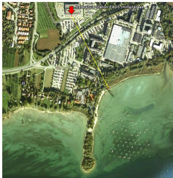
Figure 3.32: Image of the EADS facilities in Immenstaad, Bodensee. The reference station was set up on the roof with a distance to the shore of about 450m, along the drawn line.
