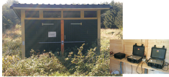
Figure 7: Hut of the permanent station. Data is recorded broad - band with two Spam IV data loggers.
