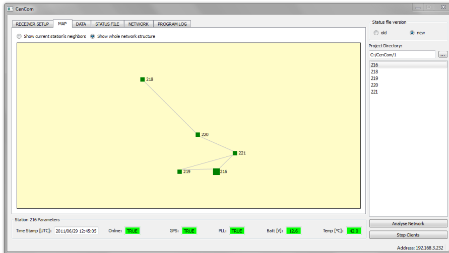
Figure 12: The central computer program. In map view all SPAM4 stations part of the mesh and their respective connections are displayed. Crucial state-of-health parameters are continuously updated in the status line (bottom of the screen) when a map symbol or the corresponding entry in the list is selected. More detailed SPAM4 information is available in the status tab.
