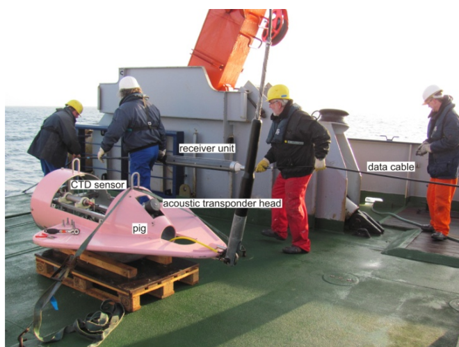
Figure 2: Deployment procedure: The CSEM system is deployed over the aft deck of the research vessel. The 'pig' an instrument platform and plough is picked up last by the A-frame and lowered to the seafloor.
