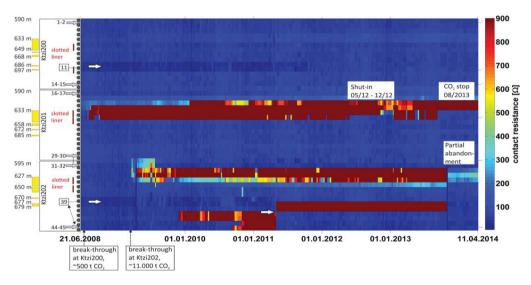
Figure 5: Update of the compact overview plot of contact resistances versus the injection history according [7], starting in June 2008 and ending in April 2014. In autumn 2013, the partial abandonment of Ktzi202 has caused as a side effect the sealing of the free annular space by overflowing cement suspension and subsequently better coupling of the electrodes along this section. The white arrows symbolize parts of the ERT arrays with gradually electrode degradation (#11, #39-#45).
