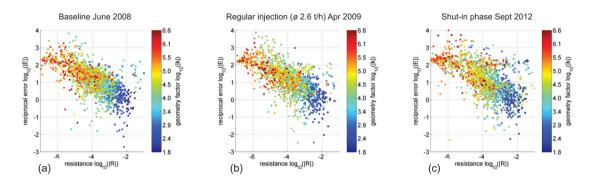
Fig. 3. Reciprocal error evaluation of the 3D field data sets, demonstrated by representative examples along the injection history: (a) baseline measurement; (b) measurement during the phase of high injection rate (~ Ø 2.6 t/h); (c) measurement during the shut-in phase which lasted from May until December 2012. Large reciprocal errors occur dominantly for configurations with large geometric factors and low measured resistances.
