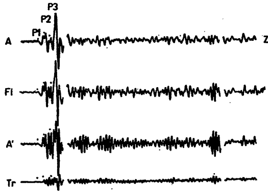
Fig. 5 Vertical records of types A, Fi, A' and Tr from an earthquake in Honshu, Japan (7 Oct 1970, D = 88.0^\circ , h = 179 km, MP1V = 5.8 , MP3V = 6.4 ).
