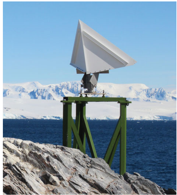
Fig. 8. (Colour online) Corner reflector at GARS O'Higgins for the ascending satellite orbit.
