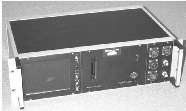
Figure 11.2.1: CAE-10-01 control and data acquisition unit
