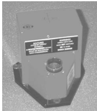
Figure 11.2.2: IGI E-Box for power and signal conversion
