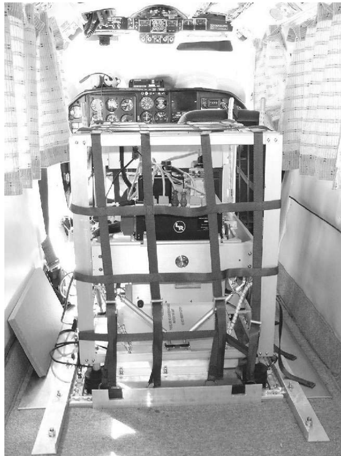
Figure 11.1.2: LaCoste & Romberg gravity meter in a Britten-Norman Islander aircraft
