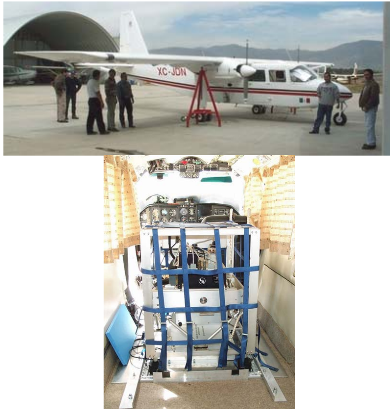
Figure 4.1: left: weight and balance inspection; right: LaCoste & Romberg gravity meter, in the rear the cockpit.
