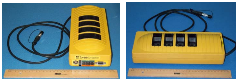
Figure 5.10: Trimble Power Unit (220 V AC to 12 V AC) and Battery Charger / Data Link (Ruler Scale is 30 cm)
