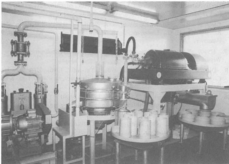
Fig. A.4.3: Automatic sampling system for cuttings and drilling fluid samples (Test phase Feb./March 1992).
