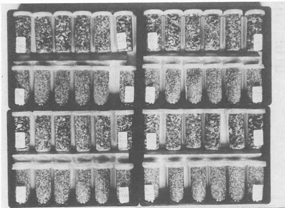
Fig. A.3.2: Example of washed, sieved and dried shaker samples (cuttings) from the uncored 4000 m of the KTB Hauptbohrung.
