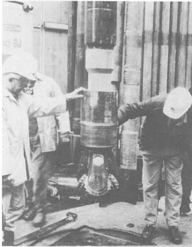
Fig. A.2.6: Junk basket (left) with an operational scheme, a prototype of a "cuttings sampler" for the 14 3/4" borehole section especially designed for use in the KTB Hauptbohrung.
