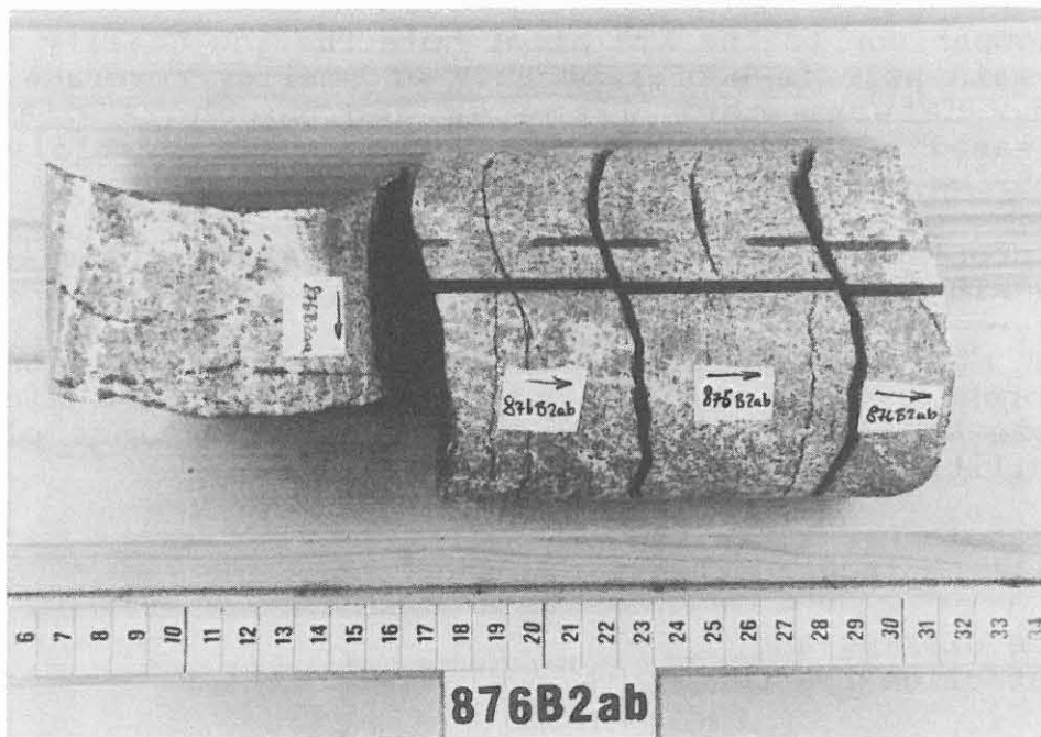
Fig. F.2: Core disking in core 876B2ab (3581.70 m).
