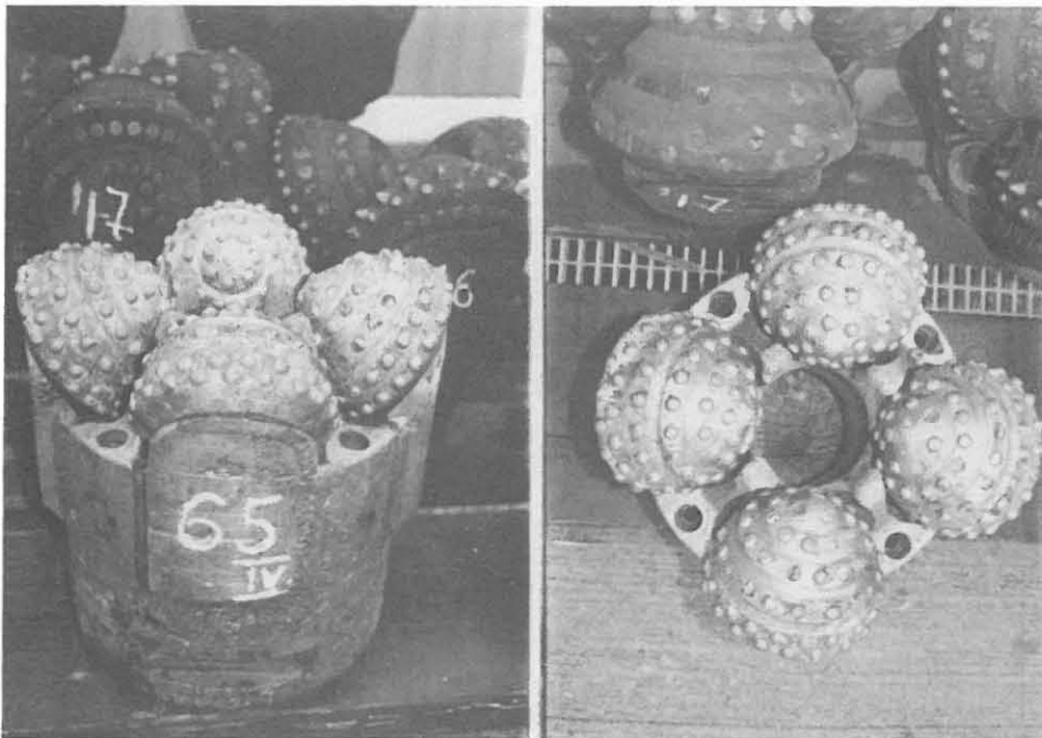
Fig. A.2.8: 14 3/4" roller cone core bits (used), yielding 4" cores.
