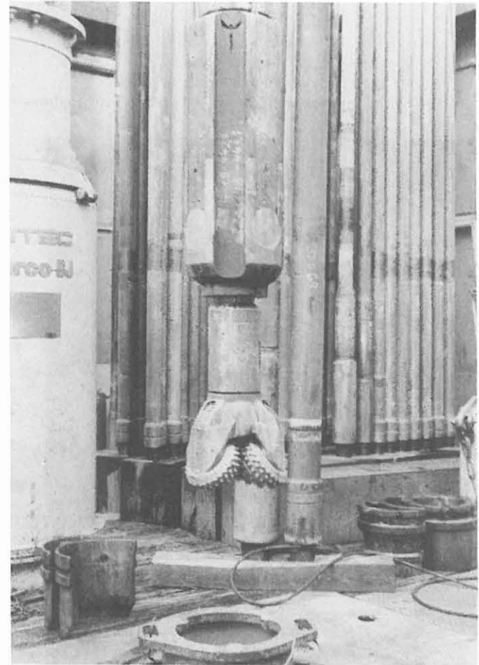
Fig. A.2.5: The active vertical drilling system VDS-3 combined with a 17 1/2" insert bit.
