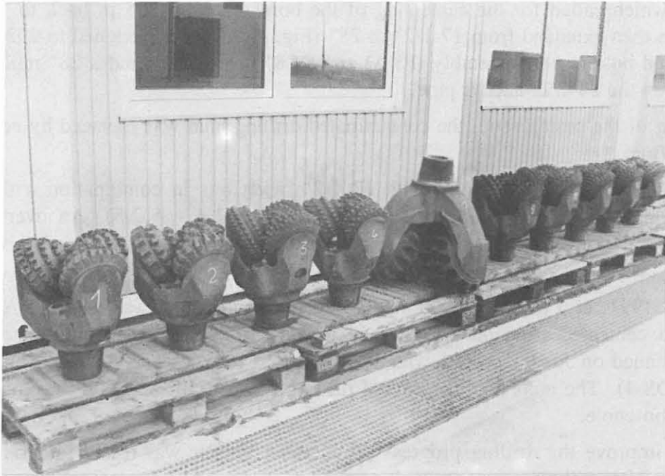
Fig. A.2.2: 17 1/2" roller cone bits used in the Hauptbohrung down to 305 m and a 28" bit used for drilling a cement plug in the 28" borehole section.
