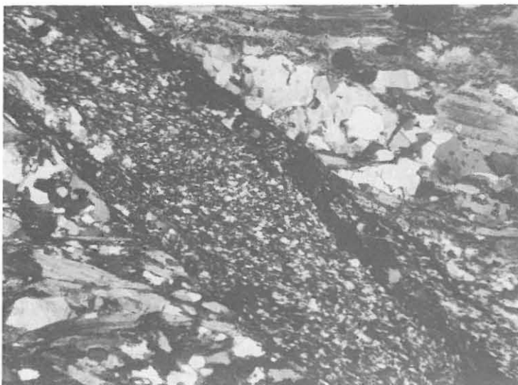
Fig. B.1 4.1.6: Discordant shearzone in paragneiss. Dynamic recrystallisation of quartz and formation of chlorite indicate deformation under greenschist facies conditions (H013B14, depth 5282 m, thinsection, crossed nicols, width of view 5.5 mm)
