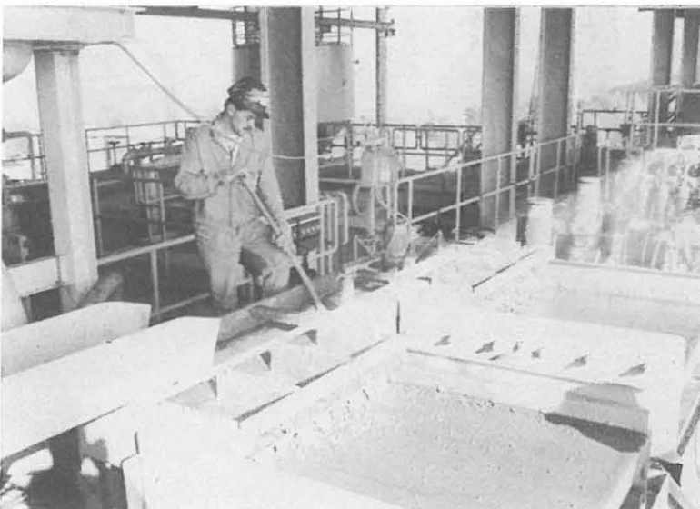
Fig. A.3.1.4: Recovery of large- sized cuttings from the possum belly in which a gas trap is installed.
