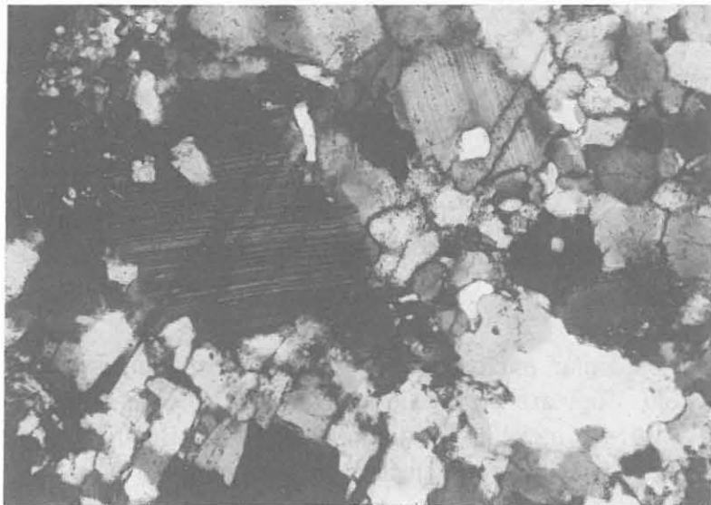
Fig. B. 2. 2.1: Subhorizontal crack sets in a bit-metamorphic amphibolite cutting (HC 3370), crossed nicols, width of view 2mm
