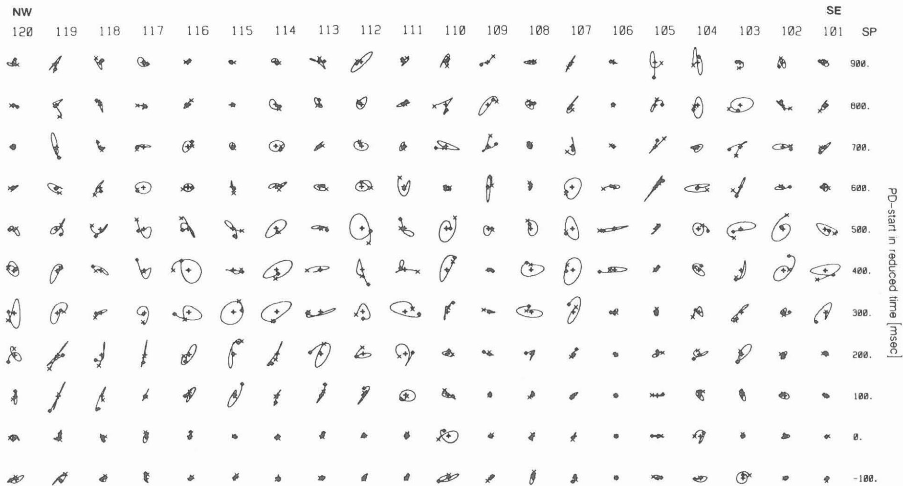
Fig. 6: Polarization diagrams in the plane normal to P-wave polarization for the recordings of the whole shot series SE of the KTB location at the geophon in 3245 m depth. The time reduction is carried out by 3.5 km/sec for the lateral offset (s. Fig. 7).
