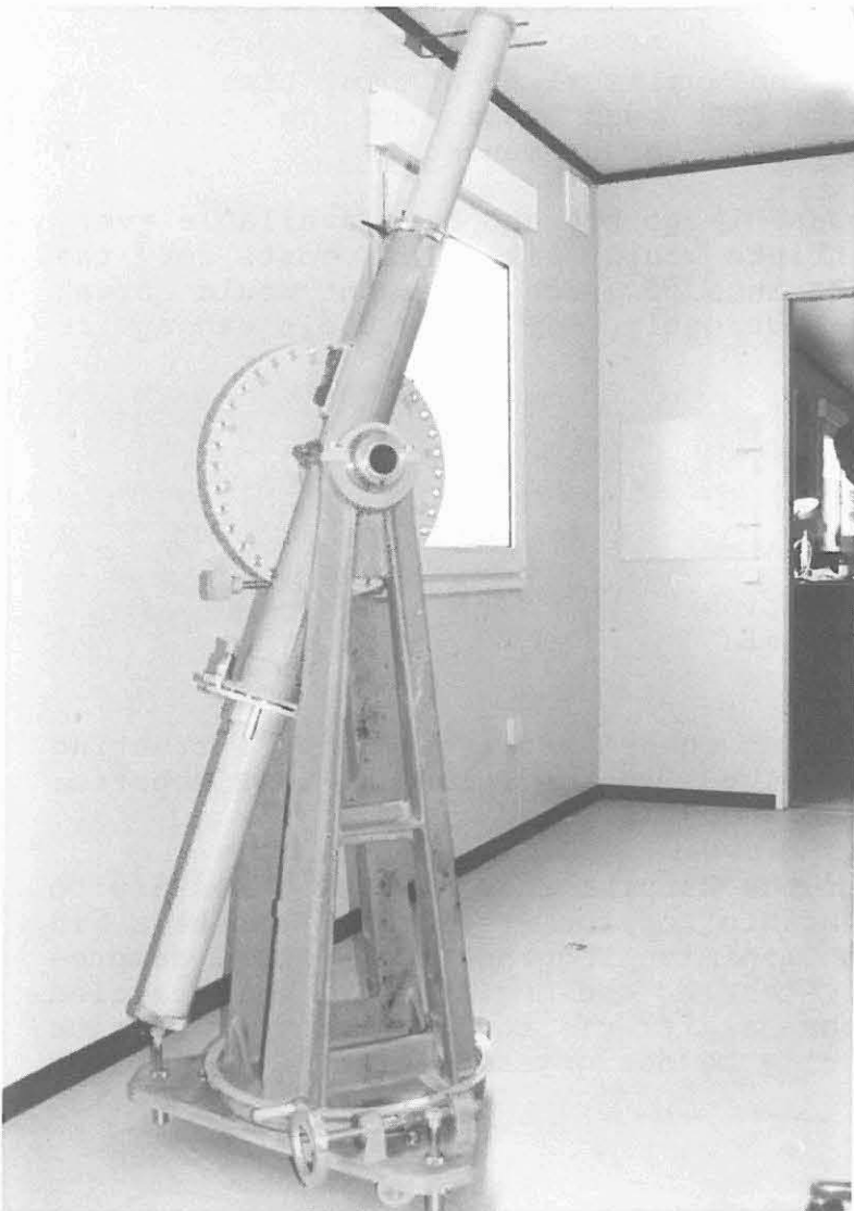
Fig. 2.24: Calibration equipment for azimuth and declination
