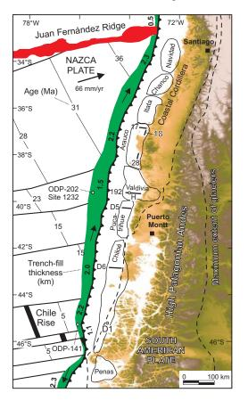
Figure 4.1: Tectonic setting of the south-central Chile margin. Forearc basins after González (1989). Nazca plate and trench-fill thickness from Bangs and Cande (1997). Maximum extent of glaciers from Rabassa and Clapperton (1990). ENAP reflection-seismic profiles discussed in the text are shown.
