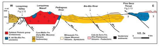
Figure 3.12: Geological cross section of the upper Bío-Bío River at ~38.5°S. The structure is controlled by the thrusting of the Mesozoic sequence over mildly deformed Oligocene-Miocene Cura-Mallín beds.
