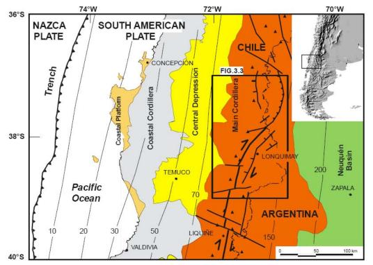
Figure 3.1: Regional location map, morphotectonic units, and Pliocene-Quaternary faults of the Main Cordillera. Contours indicate the depth to the top of the subducting Nazca plate determined using the local network seismicity from Bohm et al. (2002). Black triangles indicate Holocene volcanoes.
