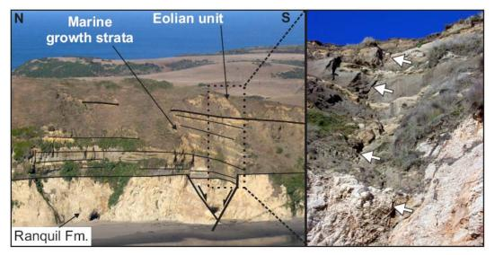
Figure B6: Oblique air photo to the east showing the northern normal fault. Note progressive upward decrease in dip of the marine unit in the hanging wall of the north dipping fault. Detail field view of a recent rupture that produced a normal offset of 0.4 m.
