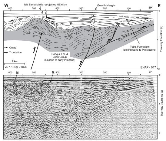
Figure 5.10: Migrated seismic reflection profile ENAP-017 (24-channel). See Figure 5.2C for location. The syntectonic sequence show eastward propagation of the deformation by footwall shortcuts. The fault below the anticline is inferred to be rooted in the plate interface area at  $\sim$ 12 km depth, which is supported by the continuous alignment of seismicity (see Figure 5.1C). M: sea-floor multiple.
