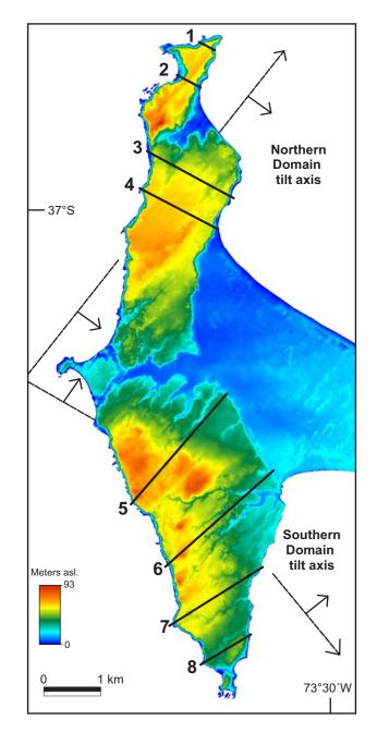
Figure B9: DEM showing location of profiles used to calculate tilting rates.
