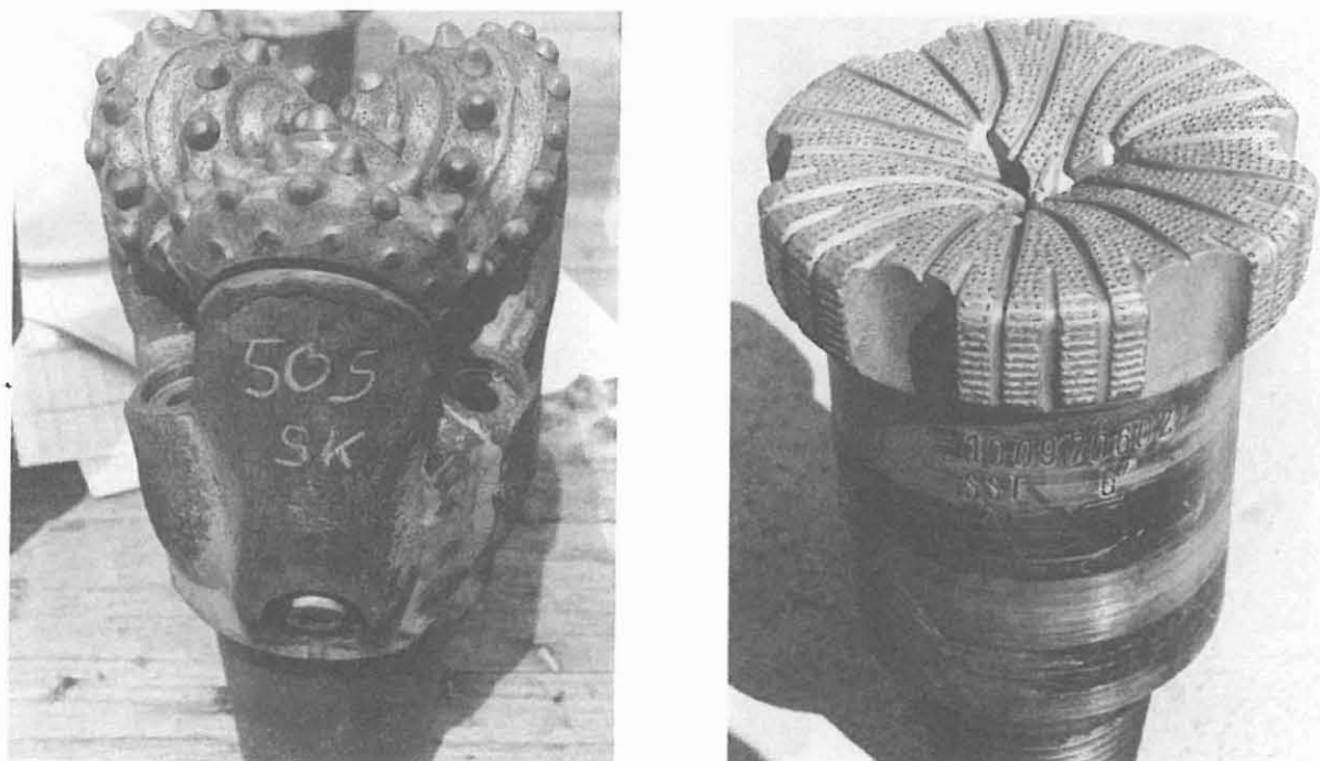
Fig. A.2.4: Two types of 6" bits used during directional drilling, roller cone bit (left picture) and surface set diamond bit (right picture)
