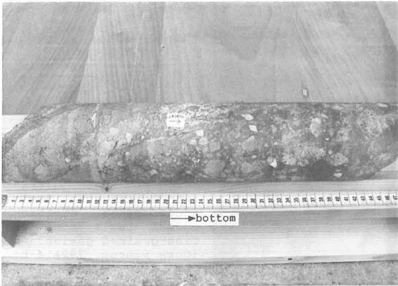
Fig. B.7.19: Fault breccia in amphibolite. Coarse-grained, angular porphyroclasts are embedded in a fine-grained matrix. (Core piece 283B1e, 1351.4 m, scale in cm).
