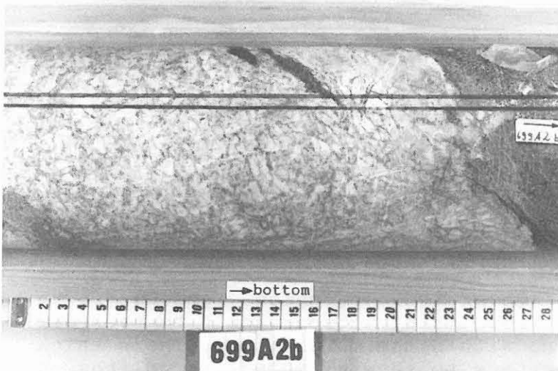
Fig. B.5.1: Quartz-plagioclase pegmatoid with biotite lenses, on the right contact to amphibolite. (Core piece 699A2b, 2858.1m, scale in cm).
