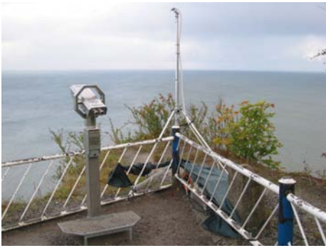
Fig. 5.3: The OpenGPS experimental setup at the Königsstuhl location with GPS patch antenna mounted on top a 2.7 m high aluminum tripod 118 m above the baltic sea-surface.
