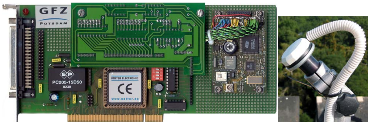
Fig. 4.1: Left: OpenGPS PCI-card with TTL logic interface board and Zarlink GPS receiver board attached. Right: Standard RHCP patch antenna mounted on a tilt- and turnable mount fixed to a geodetic tripod. The antenna is 54 mm in diameter and has a hemispheric field-of-view.
